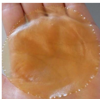
Fig.1. Chitosan film prepared by thermocompression molding using NADESs as plasticizer
